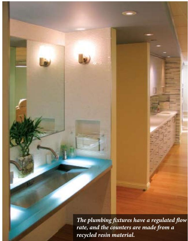
*The plumbing fixtures have a regulated flow rate, and the counters are made from a recycled resin material.*
